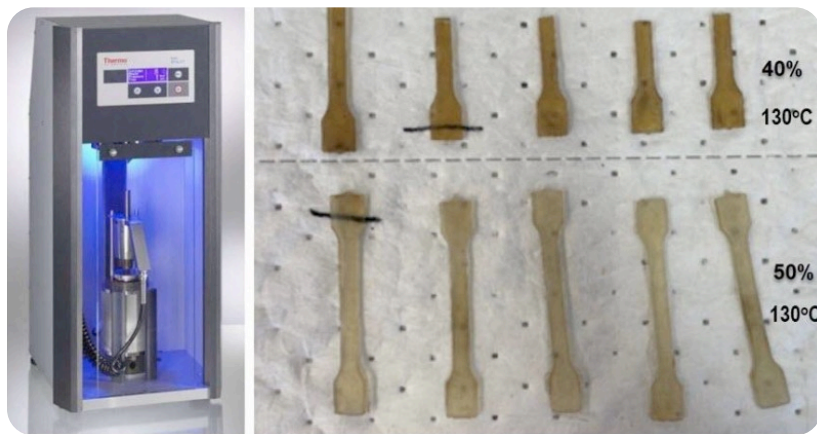
Figure 5. Thermo Scientific™ HAAKE™ MiniJet Pro Piston Injection Molding System (left) used to produce samples for mechanical property testing (right). Samples on the top row contain 40% plasticizer whereas the bottom row contained 50% plasticizer. All samples shown were extruded at 130 °C.
