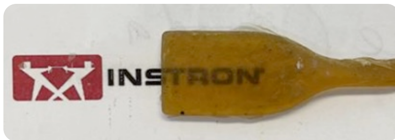
Figure 6. Transparency of a 2.95 mm thick bioplastic specimen made from 60% pea starch and 40% plasticizer.
