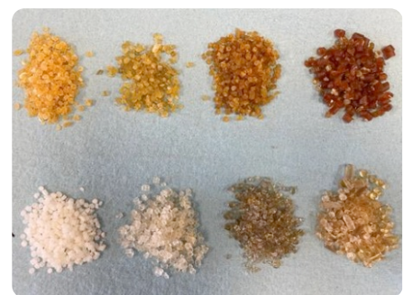
Figure 4. Pellets of pea starch bioplastics. The top row is made from starch-rich flour while samples on the bottom row are made from starch isolate.
